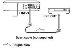
Connect the satellite or digital tuner to the LINE-3 connector as shown above.
